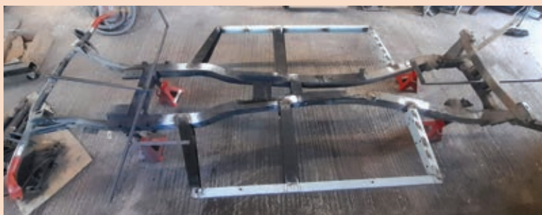
So far I have carried out some major repairs to the chassis. The main rails around the diff were particularly poor, and all the outriggers and side rails were getting crusty so were replaced.
