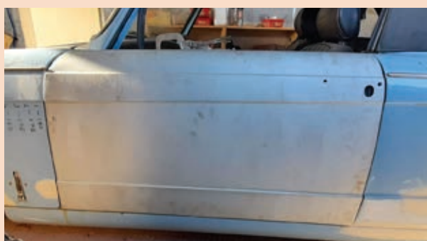
The doors have had some repairs to the frames and new skins.
