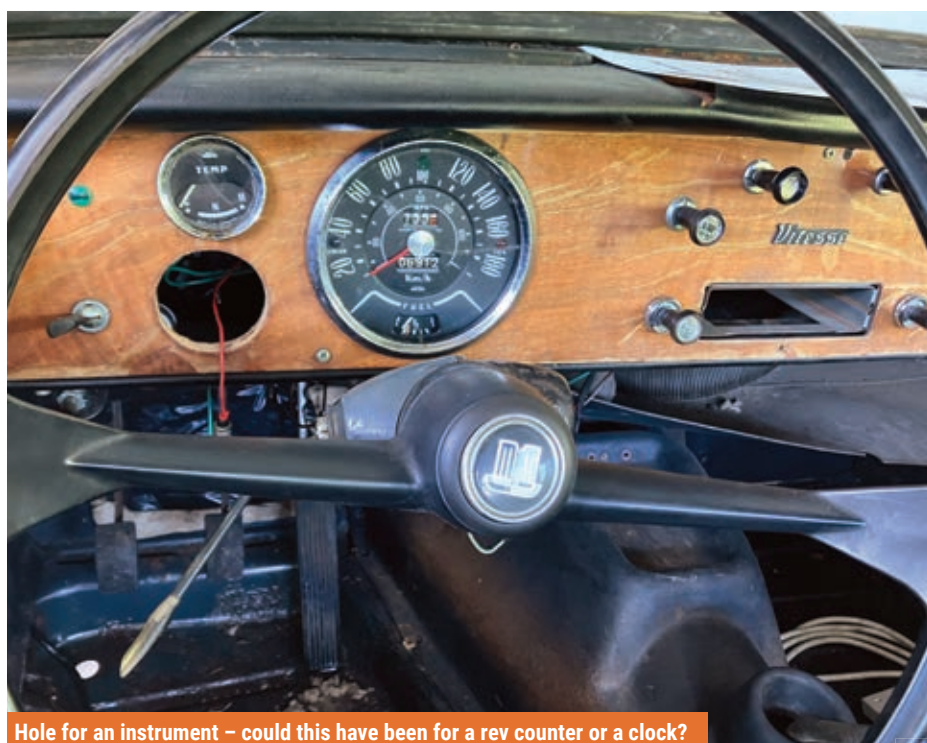
Hole for an instrument – could this have been for a rev counter or a clock?
