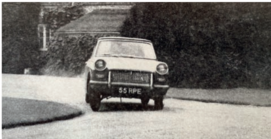
Handling characteristics are little different to the normal Herald, although the larger tyres provide rather better adhesion. Under tight cornering, oversteer quickly follows the understeer depicted here.
