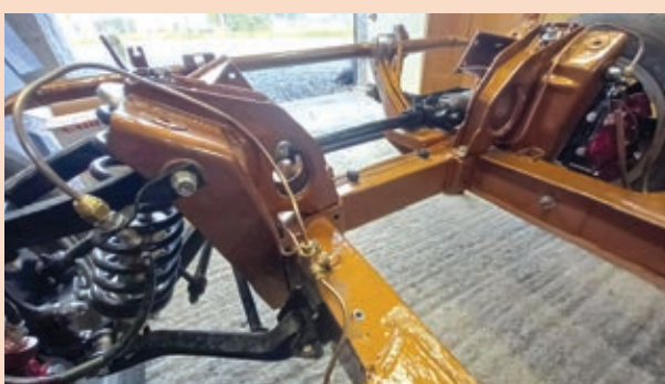
The chassis has been painted and all the suspension, brake calipers and pipes fitted so it is 'rolling'.
