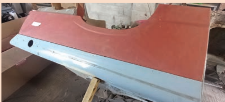
The doors have had some repairs to the frames and new skins.
