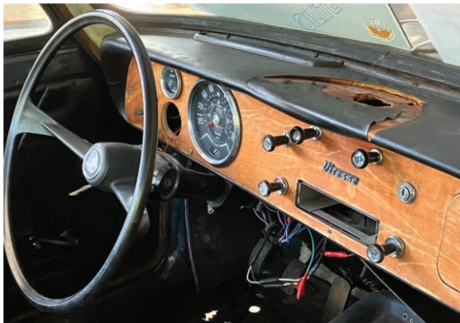
The Coupé's dashboard top has seen better days, and note typical rust hole in the footwell.
