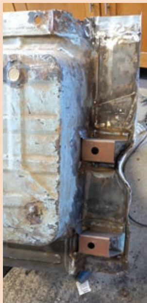
The front tub was in reasonable condition, but I fitted new body mounts and sorted out a few rusty patches underneath them.
